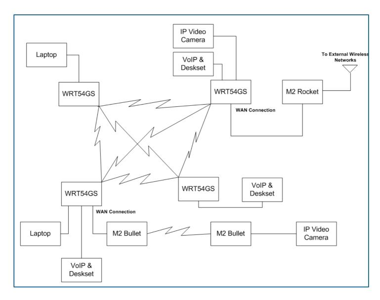
This demonstration depicts a possible configuration for an emergency network deployment during a disaster. Remote cameras can provide video back to a command center. Critical information can be transferred through the network between computers. Keyboard-to-keyboard communications can relay critical information. Full-duplex telephony – "The next best thing to being there …"
